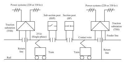
Fig. 2. Electrical principle schematic illustration of TPSSs.
