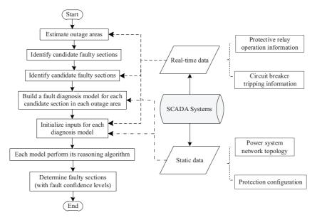
Fig. 1. Framework of fault diagnosis in power systems using reasoning model-based method.
