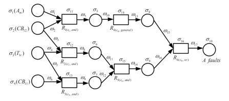
Fig. 10. A WFRSN P system fault diagnosis model for bus A.
