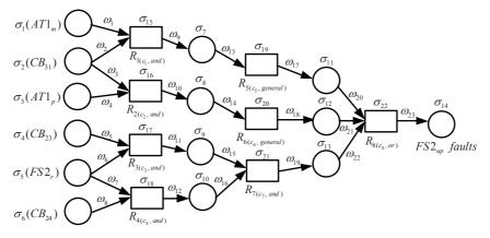
Fig. 16. A WFRSN P system fault diagnosis model for AT1.
