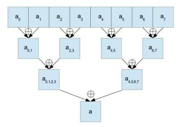
Fig. 2. Scheme of a parallel reduction solution
