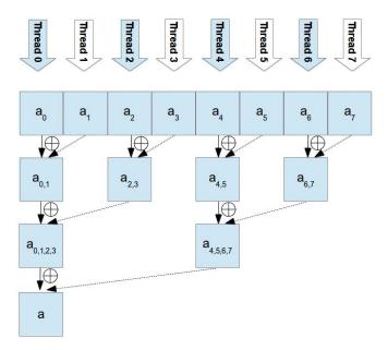
Fig. 3. Reduce0: interleaved addressing.
