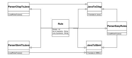
Fig. 2. Parser package: the set of classes. ParserSBMLtoJAVA identifies and recognizes the structure of the sentences according to a given grammar presented in the SBML Level 3 and build an input file in format to be read by the engine. ParserClispToJava makes the same in the inverse direction.
